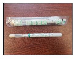
Surface samples in each crawlspace were taken at weekly intervals using HealthLink TransPorter Sterile, Sealable, Transport Swabs. Collection swabs were rubbed on a selected 4" x 4" area for 30 seconds, replaced in the collection tube, and samples kept chilled until incubated. In addition, floor joists, foundation walls, and crawlspace floors were inspected for visible signs of mold on a weekly basis.
